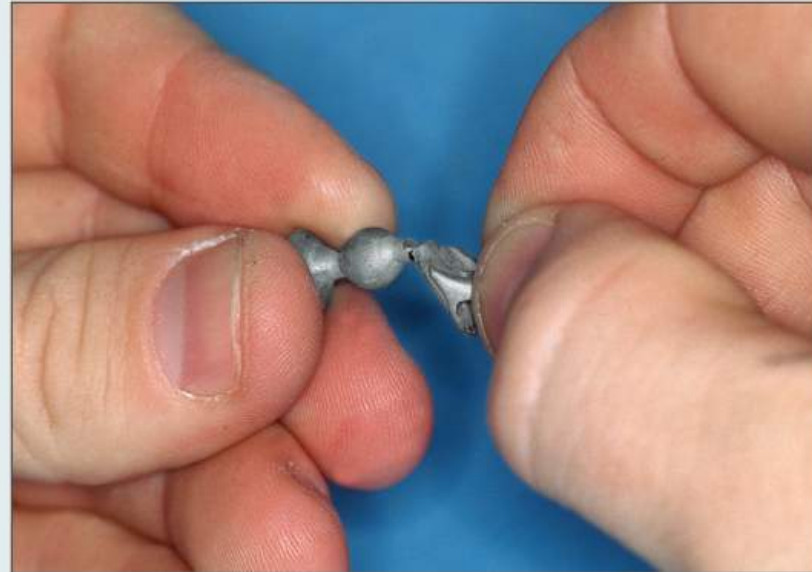
Fig 7-9b With two cuts on opposite sides, the restoration is alternately moved facially and lingually (rocked) until the coping separates from the sprue.
